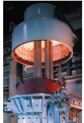
Vacuum preheating of a VIM-VIDP Crucible Furnace
